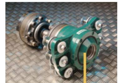
The thrust bearing is incredibly tough and built with races which can be replaced even after many years running. Sealed ball bearing races require zero maintenance on smaller Aquadrives. Taper roller units are built into the larger systems.
