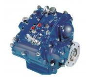
The PRM 1000 marine gearbox is purpose built for use in both pleasure craft and commercial boats; it's twin countershaft design provides separate oil-operated multi-disc clutches (which need no adjustment) for ahead and astern drive allowing full rated power to be transmitted continuously in either direction.
