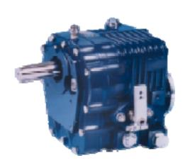
The gearbox is purpose built to operate with standard rotation engines i.e. providing a clockwise rotation of the gearbox input shaft when viewed on input. In forward drive the output shaft rotates opposite to input shaft therefore requiring a right hand propeller. The reduction ratios offered are 2.04:1 and 2.94:1 with a common astern ratio of 2.5:1.
