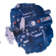
The reduction ratios offered (1.53:1, 2.09:1 and 2.82:1) are all available for left-hand or right-hand propeller rotation, making the PRM 150 particularly well suited to twin engine installations. The heavy duty aluminium gear case is externally ribbed for rigidity & strength and consists of two separate halves to facilitate servicing.
